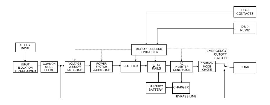
FIGURE 1: S SERIES BLOCK DIAGRAM
