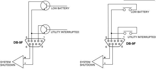
SIGNAL: OPEN-COLLECTOR CONTACT CONNECTOR
