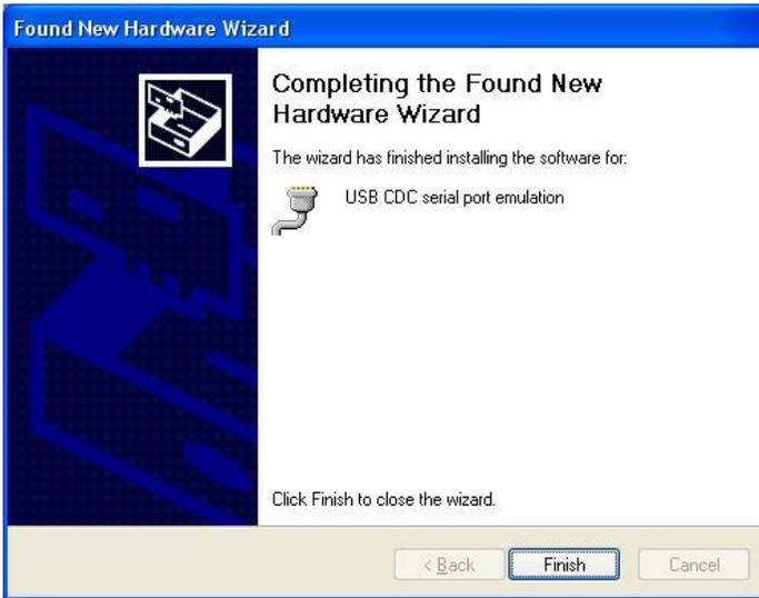
9. Go to your device Manager, then click on the “Ports (COM & LPT)” tab. You will see the USB CDC serial port emulation (Com 1, 2, 3...etc.). This will be the com port assigned to your USB port. This is the Com port you will use when connecting to the Clary Software while using the USB port.
