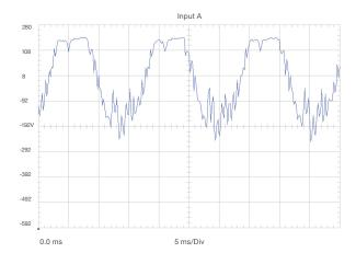
This image shows the output from a portable generator. The sinewave is erratic. But when the generator output is run through a Clary UPS, the wave form is corrected and stable sinewave output is sent to power your equipment.
